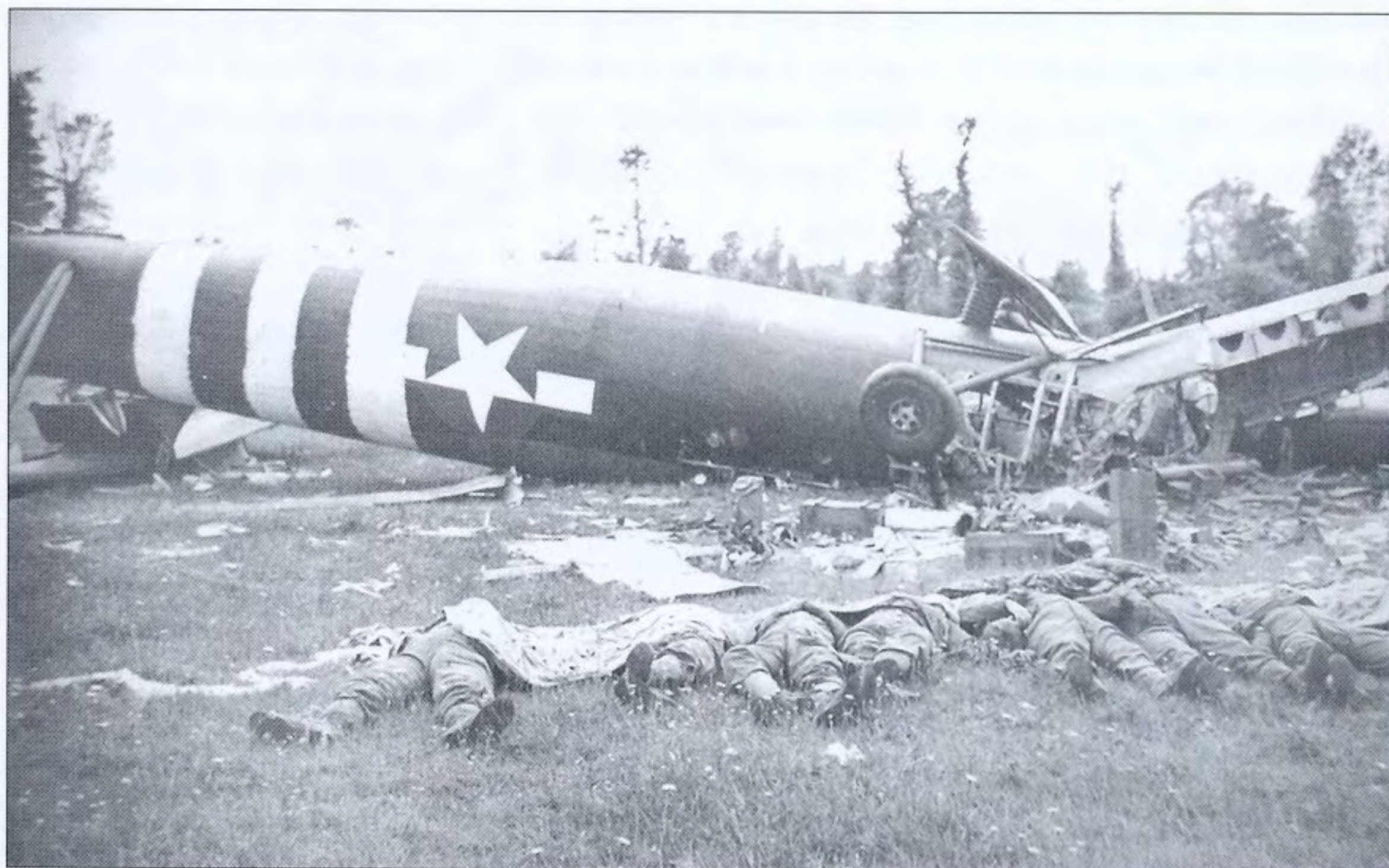
The inherent dangers of glider transport took their share of lives; here dead troopers of the US 101st Abn Div lie by a flipped-over Waco CG-4A. Gliders could be wrecked on landing by natural or man-made obstacles, or by flipping if the wheels jammed into soft ground (many gliders jettisoned their take-off wheels and landed on skids). The Waco could carry 15 men; the US Army also used a number of Horsas for their larger capacity.
