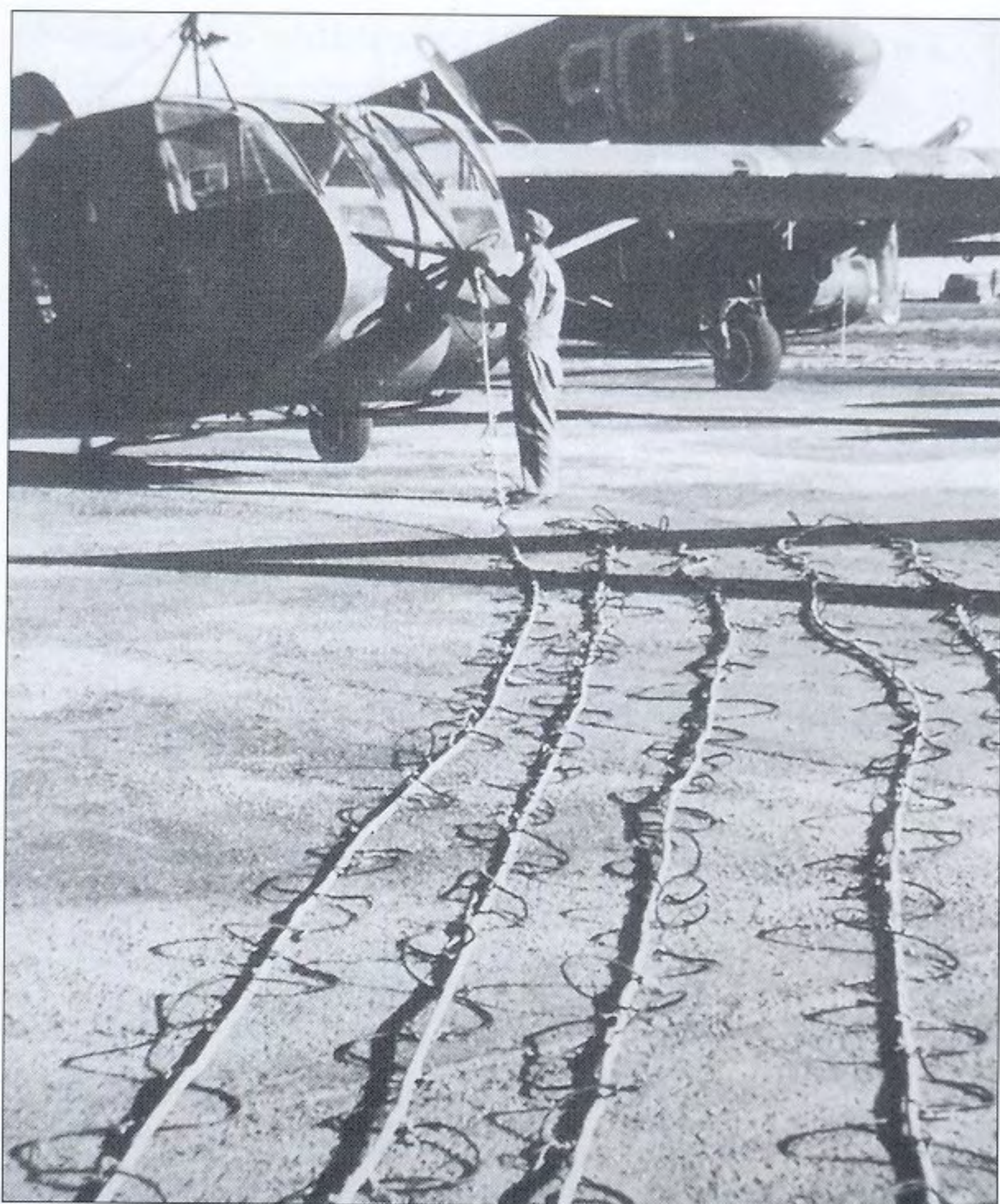
Here a ground crewman double-checks the towrope release on a Waco CG-4A glider. The ropes are laid out in a 'S'- pattern to pay out smoothly as the tug takes off. The telephone intercom wire linking the pilots of the glider and its C-47 tug can be seen taped to the towrope in a manner that allowed for rope stretch.
